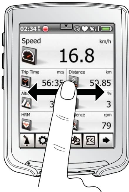
**Figure 6. Switching between bike computer and map mode**
